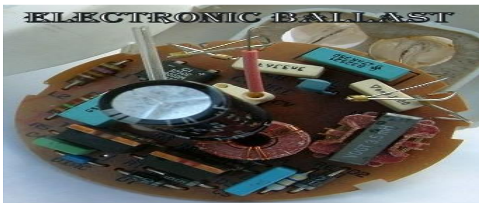
Figure-1 Electronic ballast of CFLs
